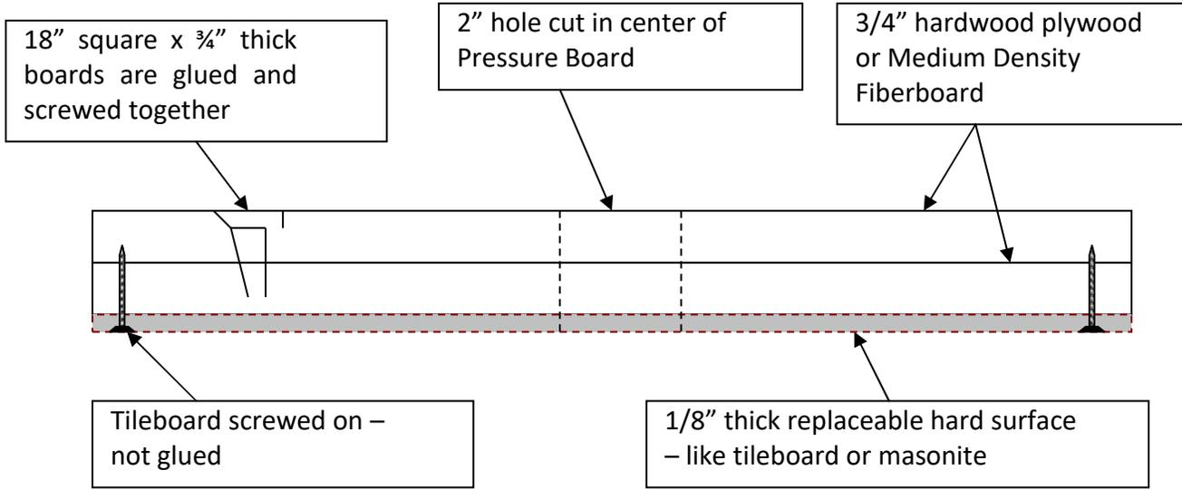
**Figure 2 – top view of Pressure Board**
